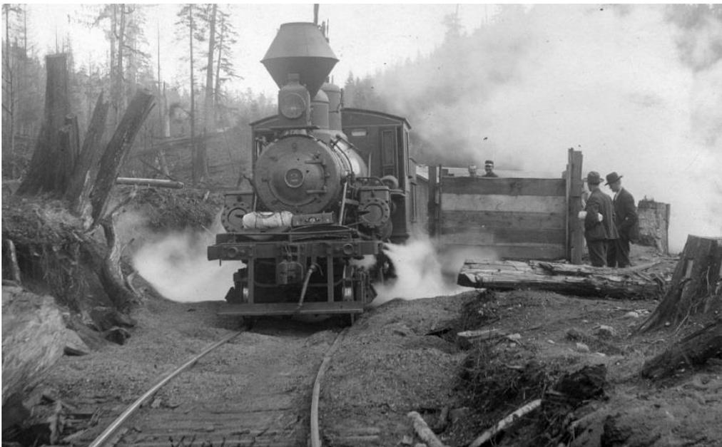
Another type of logging locomotive common in the Northwest was the Climax, characterized by two cylinders, mounted at an angle fore-and-aft, one on each side of the engine. Sobeys Mfg Co., later Waite Mill, operated a Climax locomotive, shown here being refueled near the mill.
