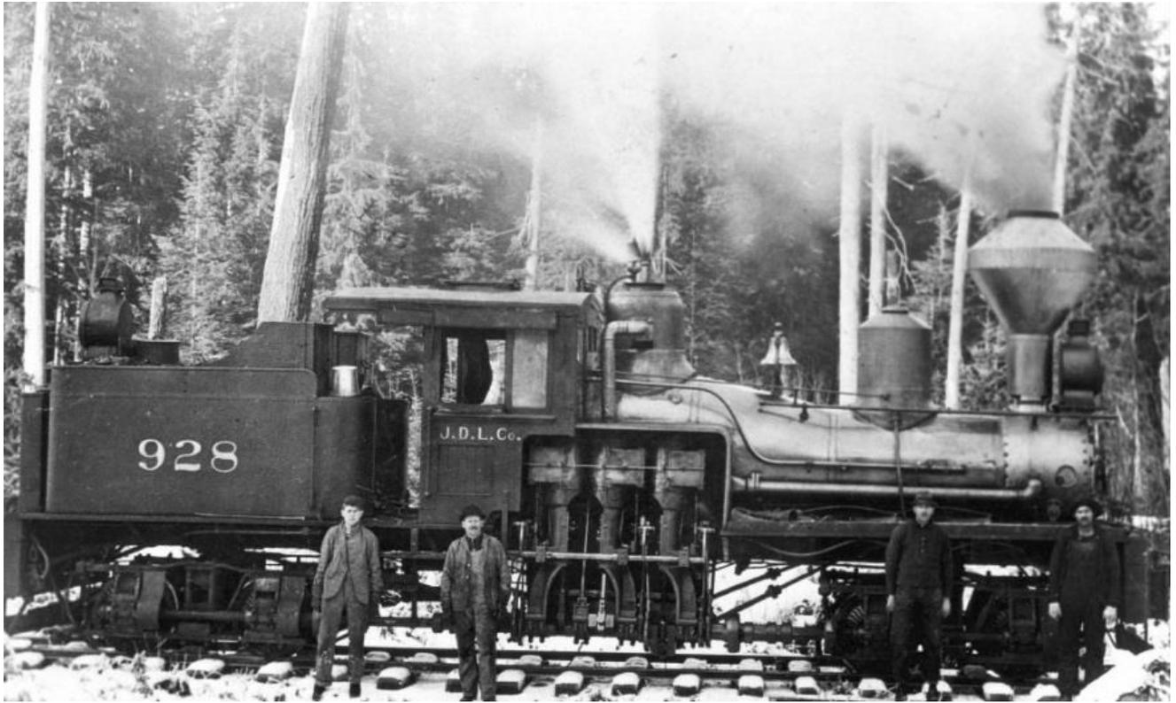
Most Shay locomotives sported three vertical cylinders, placed on one side, and had a long boiler that was offset from the centerline of the engine. Some had two “trucks” (sets of wheels) like #928, and some had three, carrying extra-large loads of fuel. The drivelines and universals were a mechanical marvel.
